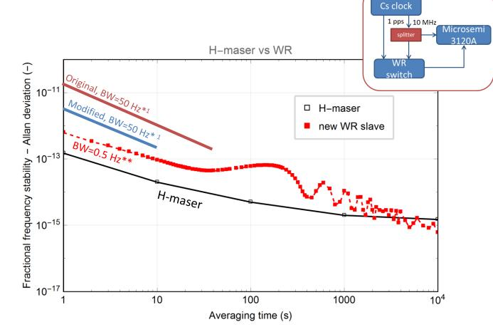
\*bandwidth (BW) of microsemi 3120A is set to 50 Hz \*\*BW of microsemi 3120A is set to 0.5 Hz. This affects the level of the Allan deviation curve. A bandwidth of 0.5 Hz is used for long term measurements to decrease the amount of data. This immidiately shows what a clean-up oscillator with a phase lock bandwidth of ~0.5 Hz would do.
